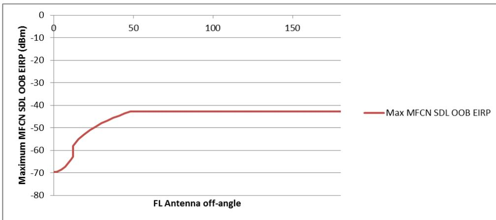
**Figure 12: Maximum MFCN SDL Base Station Station out-of-band e.i.r.p. as a function of the Fixed Link antenna off angle, for MFCN SDL vs uncoordinated Fixed Link scenario**
