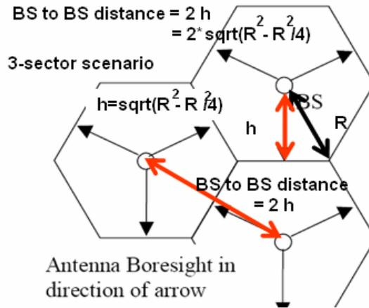
**Figure 16: Network layout and cell radius definition**
