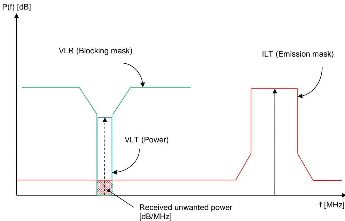
**Figure 18: Wanted signal and Unwanted emissions**
