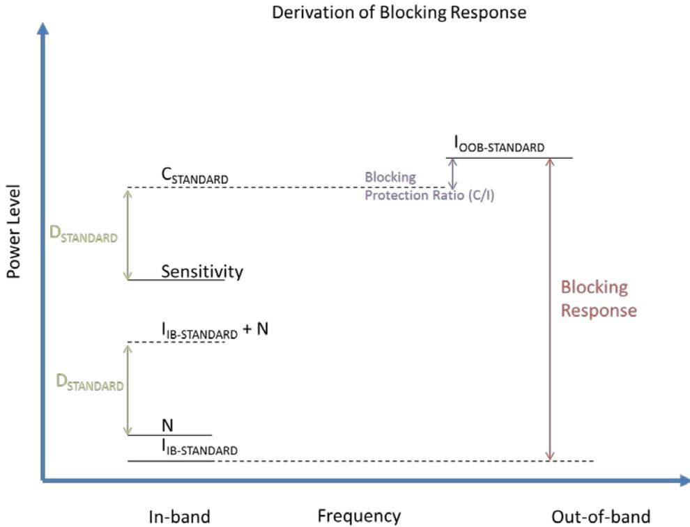
**Figure 17: Derivation of the Blocking Response for standard providing a Blocking Protection Ratio**
