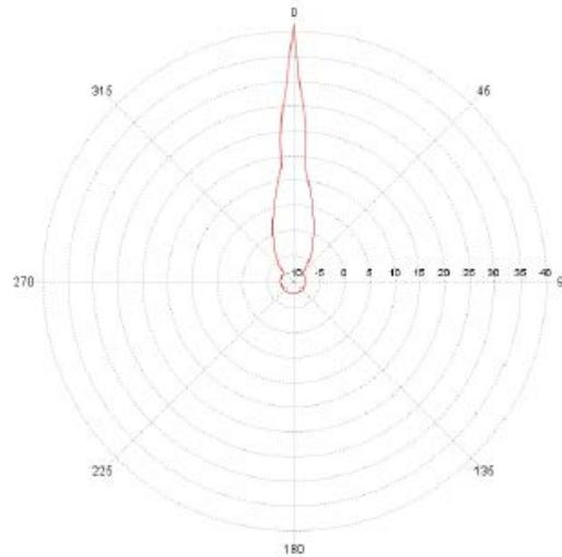
**Figure 5: Aeronautical System Antenna Pattern given by Recommendation ITU-R M.1459**
