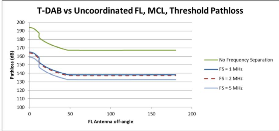
**Figure 10: Threshold Pathloss for coexistence between T-DAB and Uncoordinated Fixed Link**
