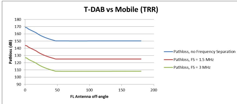
**Figure 11: Threshold Pathloss for coexistence between T-DAB and Tactical Radio Relay**
