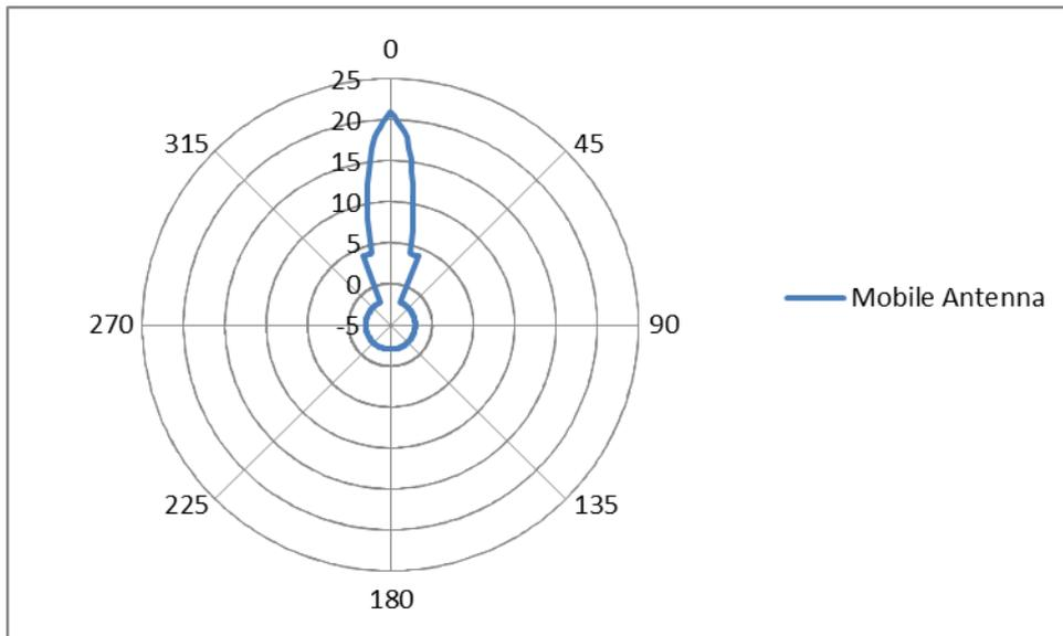
**Figure 4: FS antenna patterns for Tactical Radio Relay, where Maximum Gain = 21 dBi**
