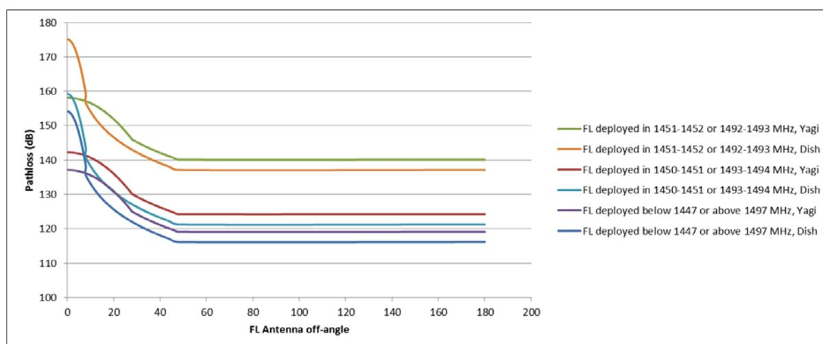
**Figure 6: Path loss between MFCN SDL Base Station and Fixed Link Station under which coordination is required**
