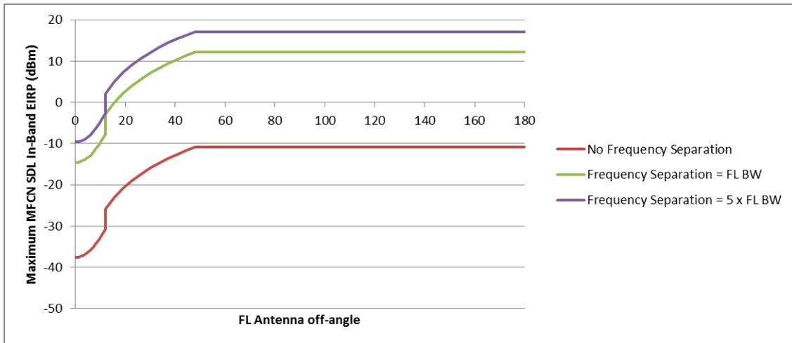
**Figure 13: Maximum MFCN SDL Base Station in band e.i.r.p. as a function of the Fixed Link antenna off angle, for various Frequency Separations, for MFCN SDL vs uncoordinated Fixed Link scenario.**
