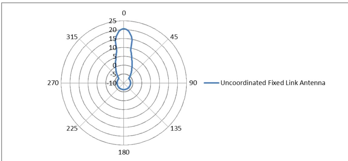
**Figure 3: Antenna pattern for uncoordinated Fixed Links**
