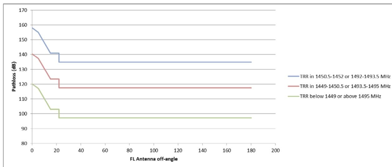
**Figure 7: Path loss between MFCN SDL Base Station and TRR Station under which additional interference mitigation techniques are required**
