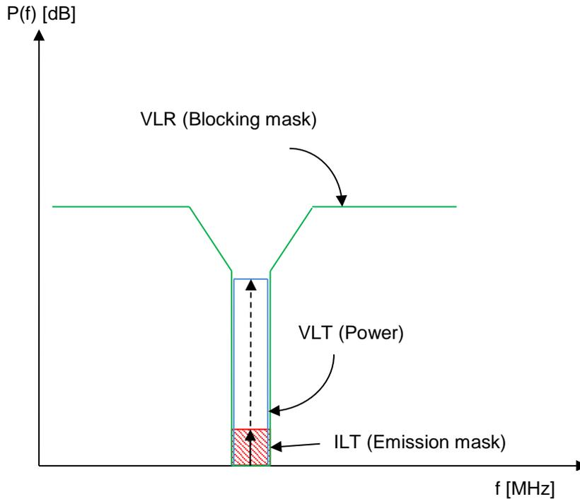
**Figure 19: Simplification of coexistence analysis**
