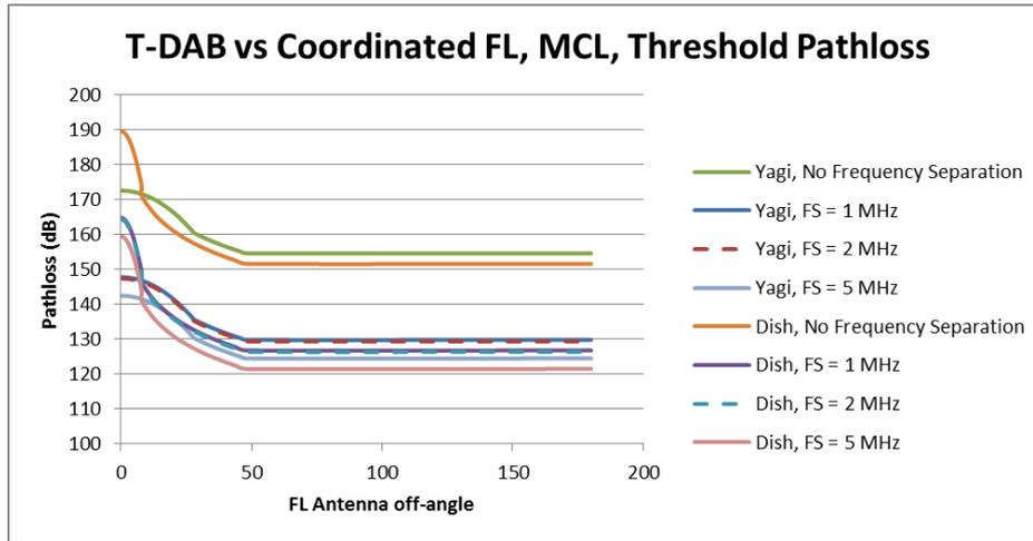
Figure 9: Threshold Pathloss for coexistence between T-DAB and Coordinated Fixed Link
