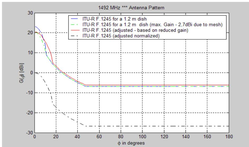
**Figure 14: Antenna Pattern based on ITU-R F.1245-2 [9]**
