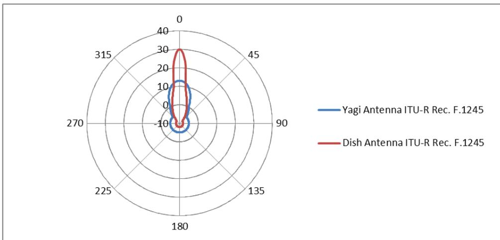
**Figure 2: FS antenna patterns derived from ITU-R Rec. F. 1245**
