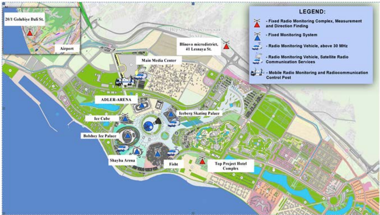
Figure 6: Arrangement diagram of the Sochi 2014 Automated Radio Monitoring System elements in the territory of the Coastal Cluster
