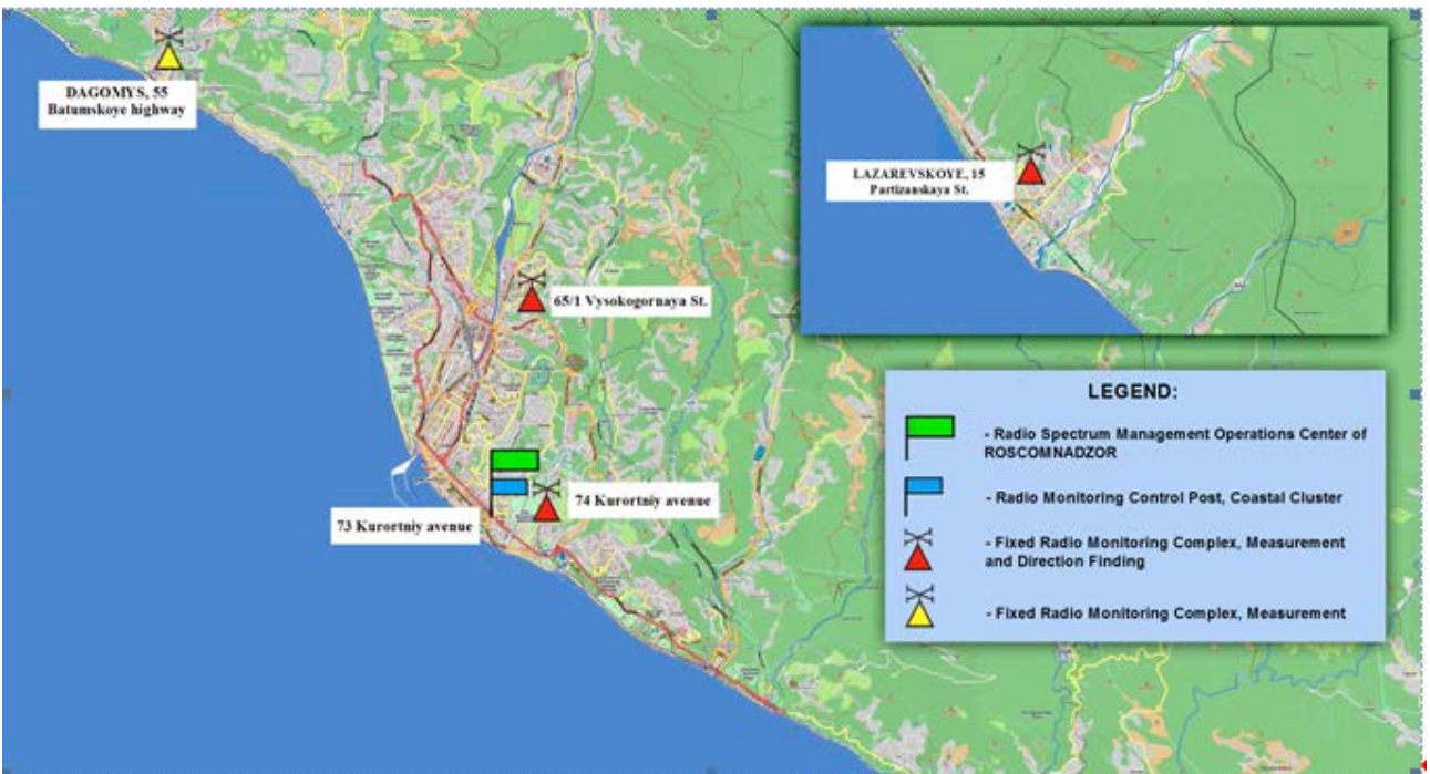
Figure 5: Arrangement diagram of the Sochi 2014 Automated Radio Monitoring System elements in the territory of the Greater Sochi
