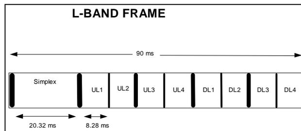
Figure 3: IRIDIUM Frame Structure
