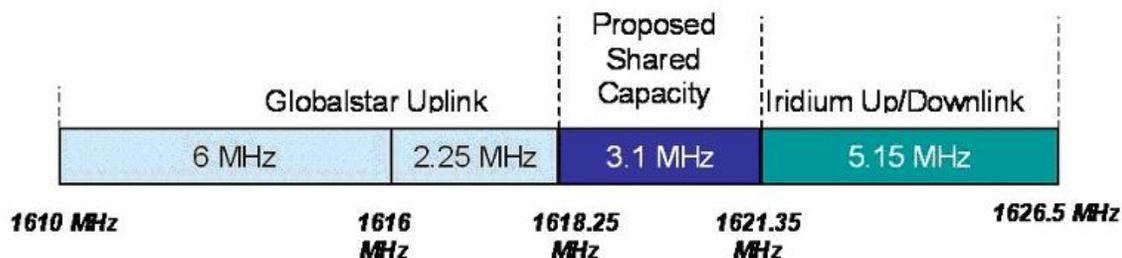
Figure 1: Proposed usage of the MSS allocation between 1610 and 1626.5 MHz
