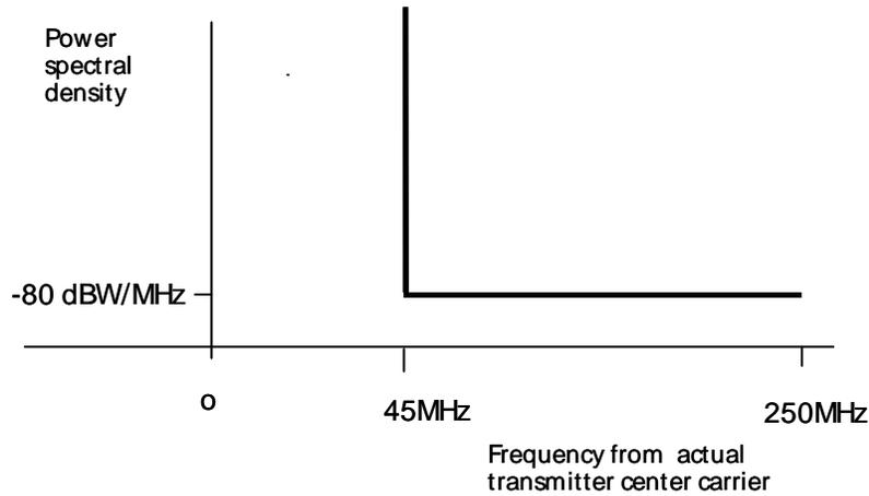
**Figure 12: Limits of spectral power density for 100 MHz radio channels (ETSI EN 300 408)**
