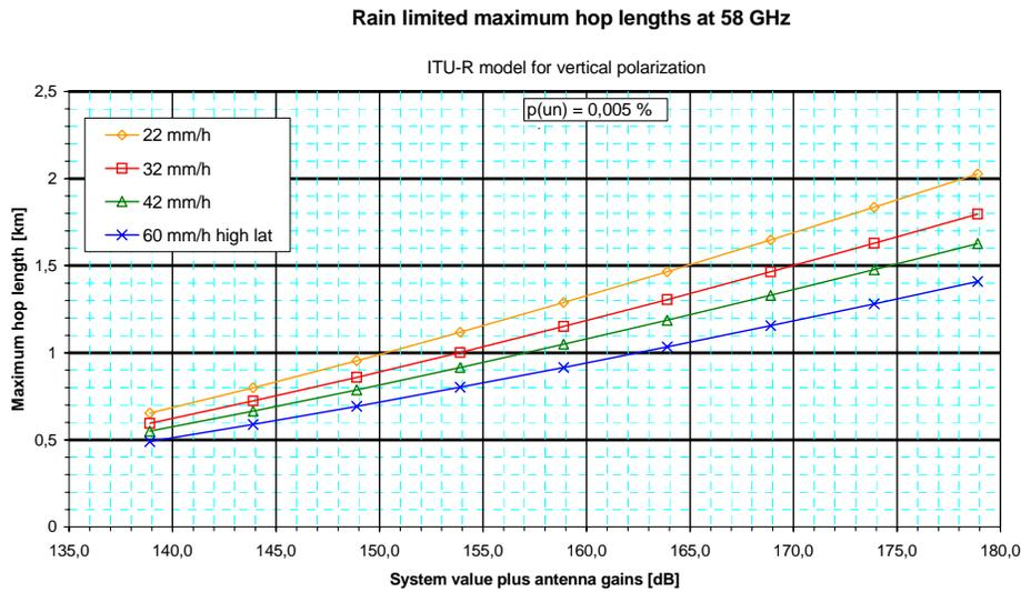
Figure 1: Maximum hop lengths vs. System Gain
