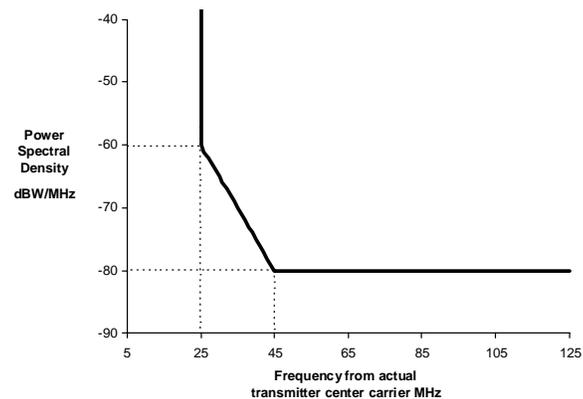
**Figure 11: Limits of spectral power density for 50 MHz radio channels (EN 300 408)**
