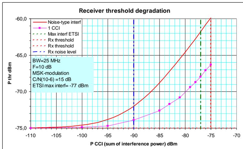
**Figure 2: Receiver threshold degradation**
