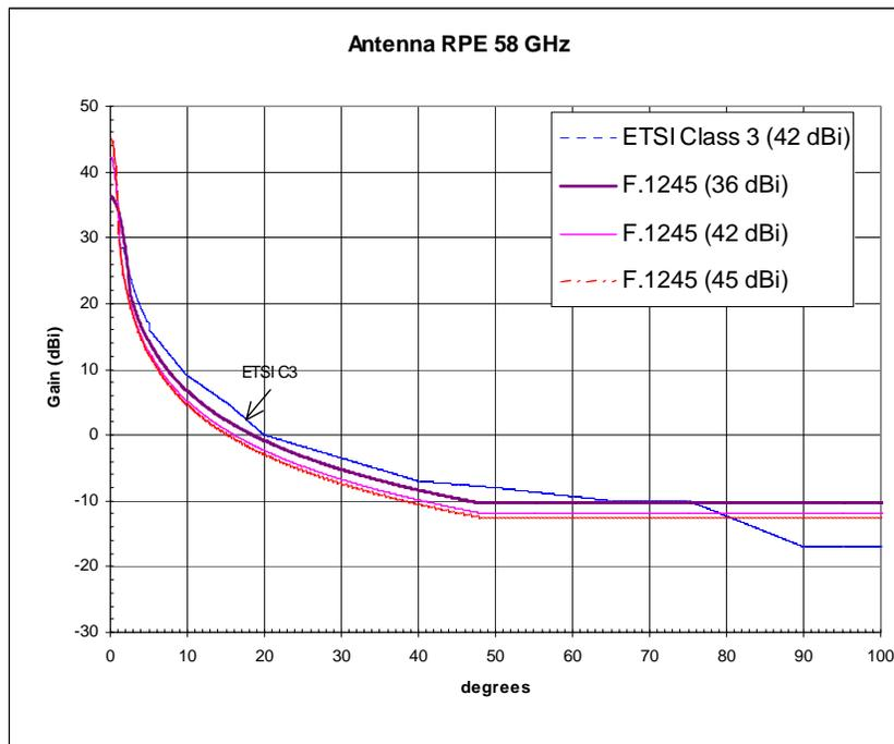
**Figure 3: Antenna RPE curves for antennas used in the intra-band interference calculation (ETSI Class 3 RPE only for reference)**
