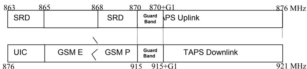
**Figure 1: SRD and TAPS systems around 870 MHz**
