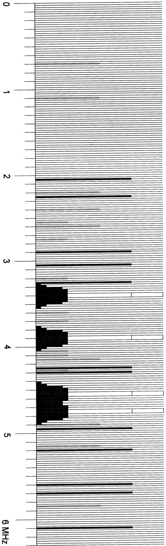
**Set 4 4 Channels. Showing intermodulation products**
