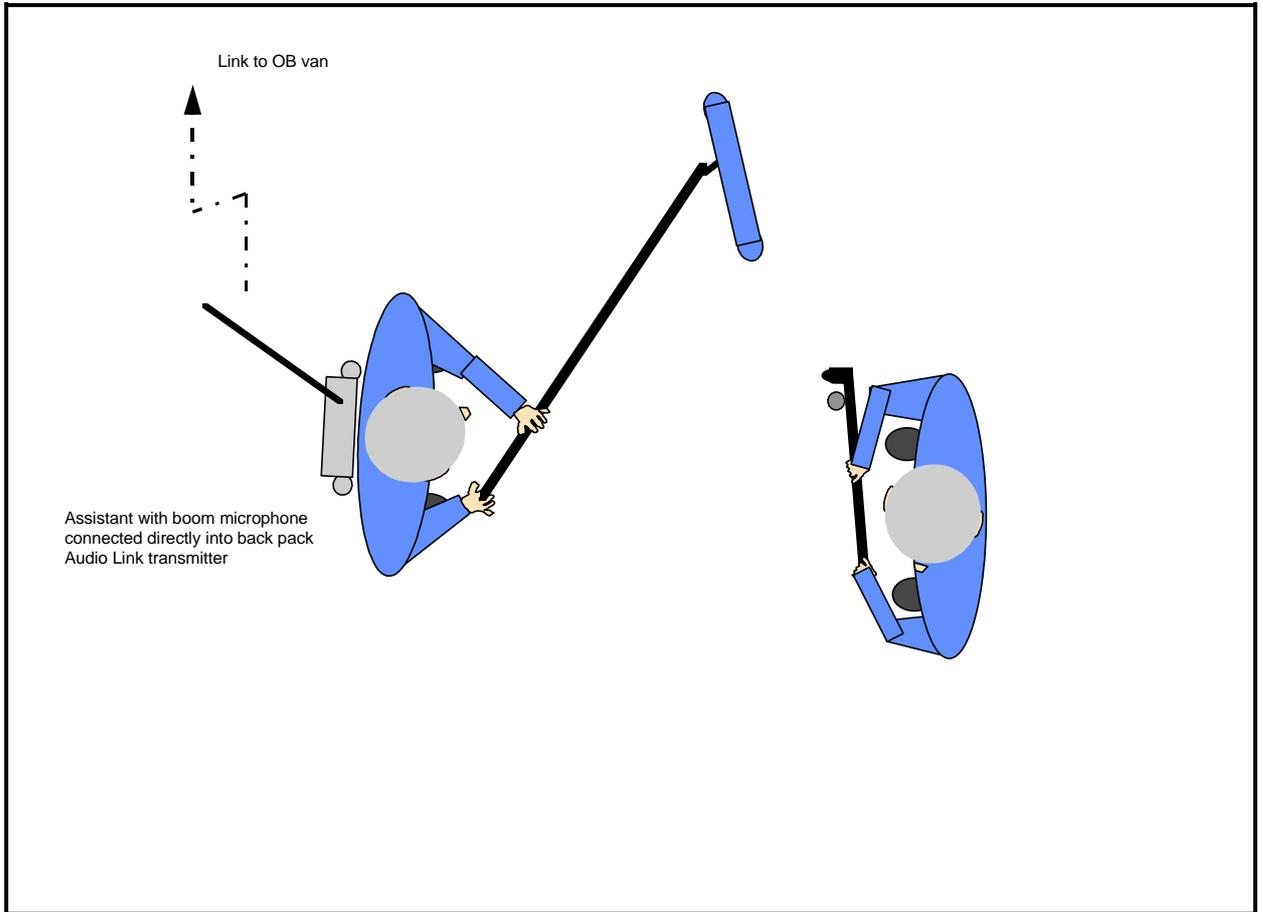
Figure 5: Location sound (Direct feed from microphone to link transmitter carried by a sound assistant as a backpack)
