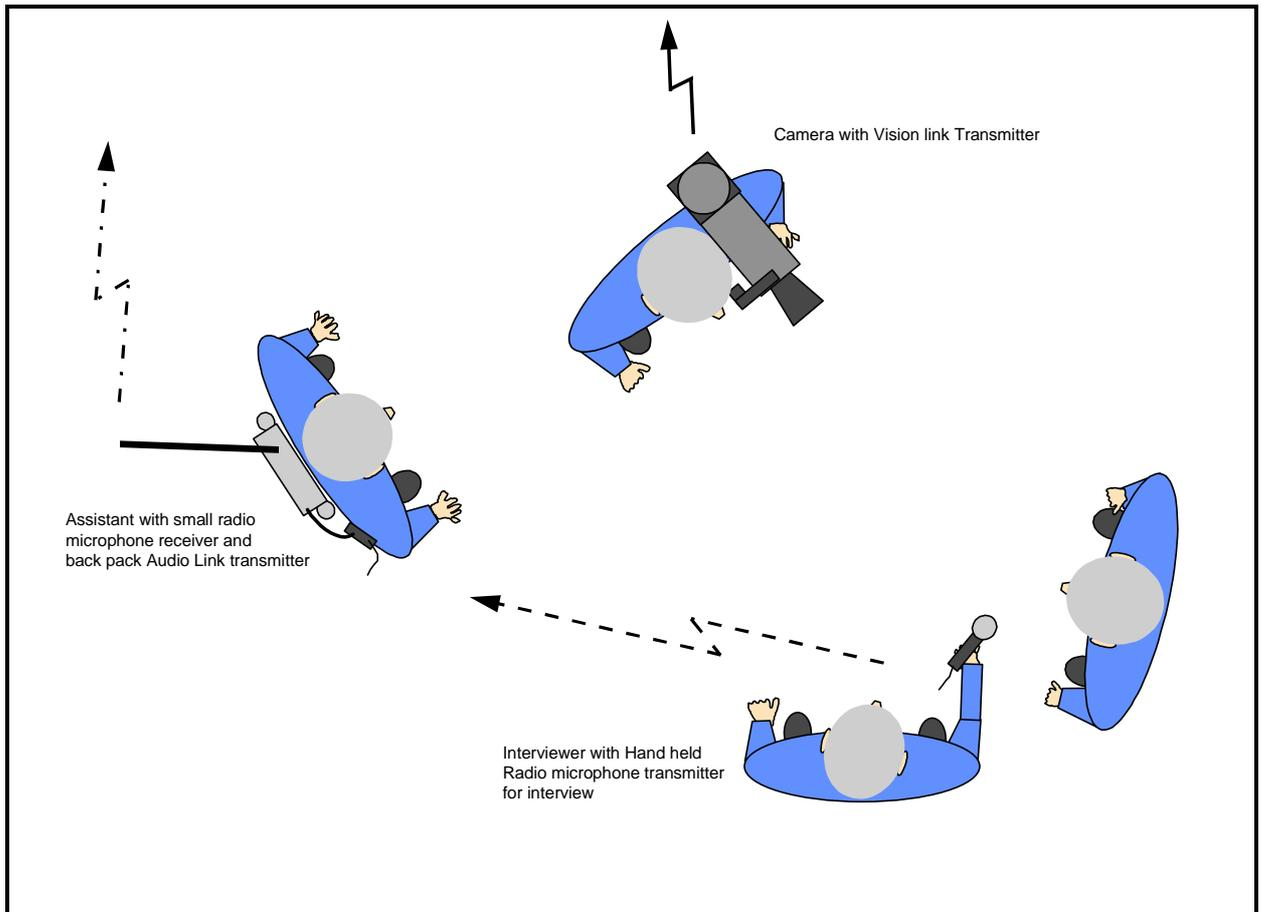
Figure 4: Interviewer to assistant, link to OB van (1 handheld transmitter, 1 small receiver, 1 link transmitter)
