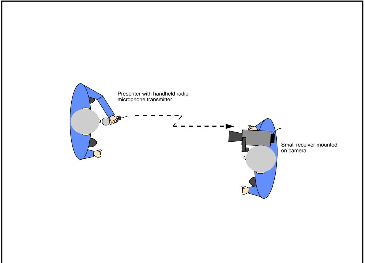
Figure 1: Reporter to camera (handheld transmitter, small camera mounted receiver)
