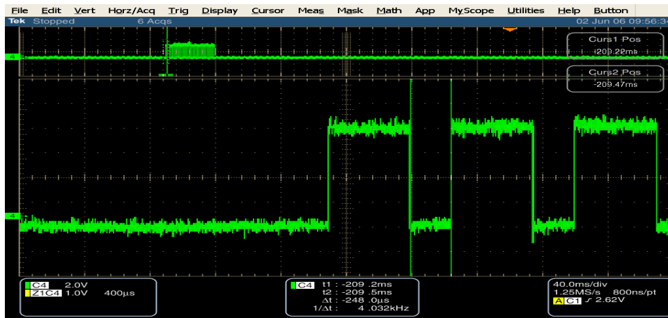
Figure A2.5 : Zoom of A2.corresponding to the 500 µs / 250 µs sequence
