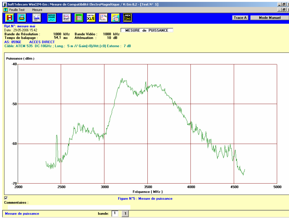
Figure A3.3: Measurement of Wimax Downlink
