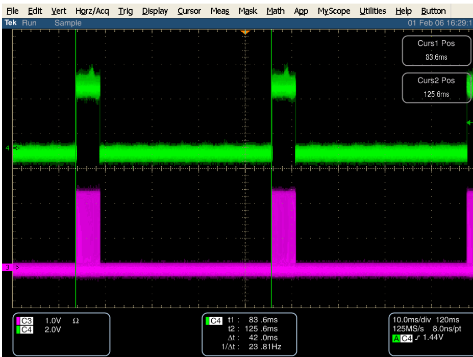
Fig A2.2: Ton 5 ms and Toff 38 ms
