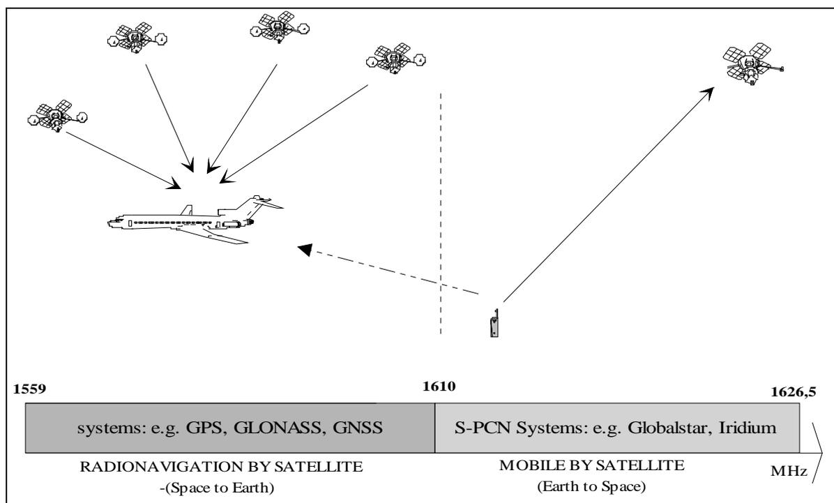
**Figure 1: Sharing situation in adjacent bands between MSS and RNSS**
