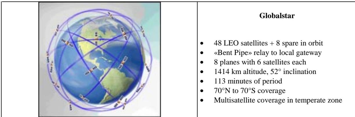
**Figure 2: Typical MSS system**
