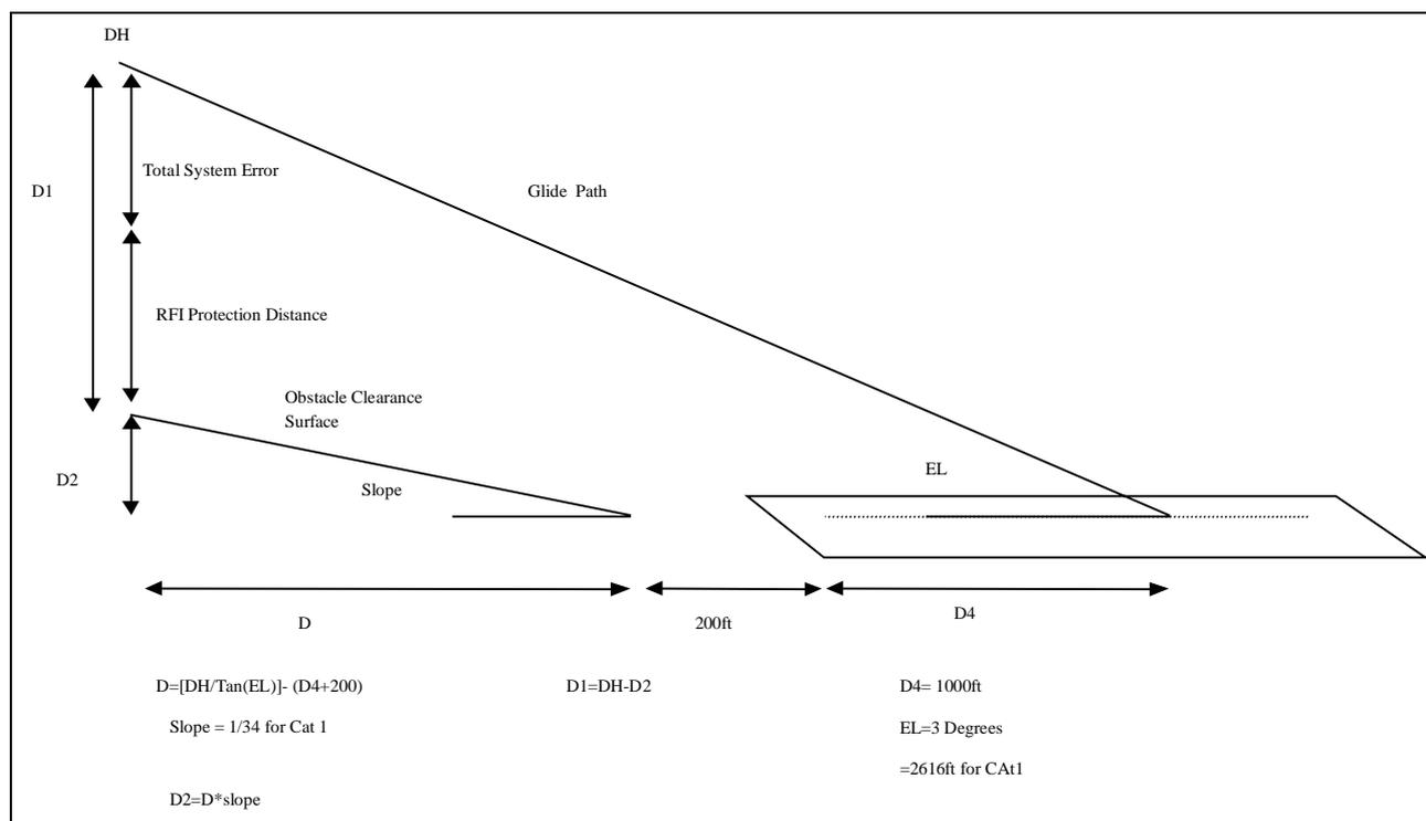
**Figure 5: Distance between MES and RNSS receiver**
