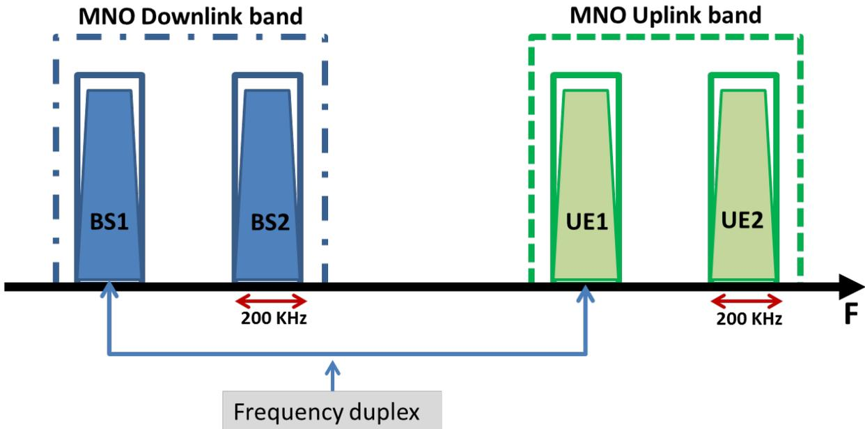
Figure 3: Standalone deployment of IoT
