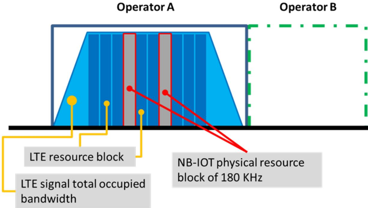
Figure 2: In-band deployment of IoT
