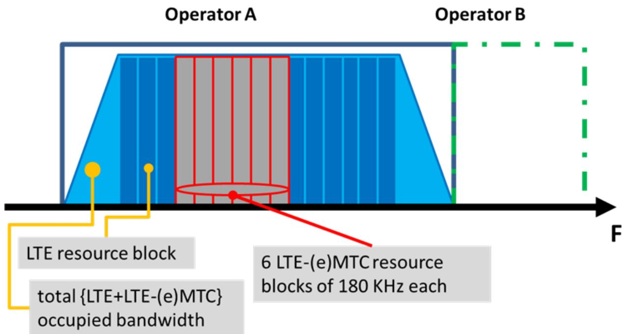
**Figure 1: In-band deployment of LTE (e)-MTC**
