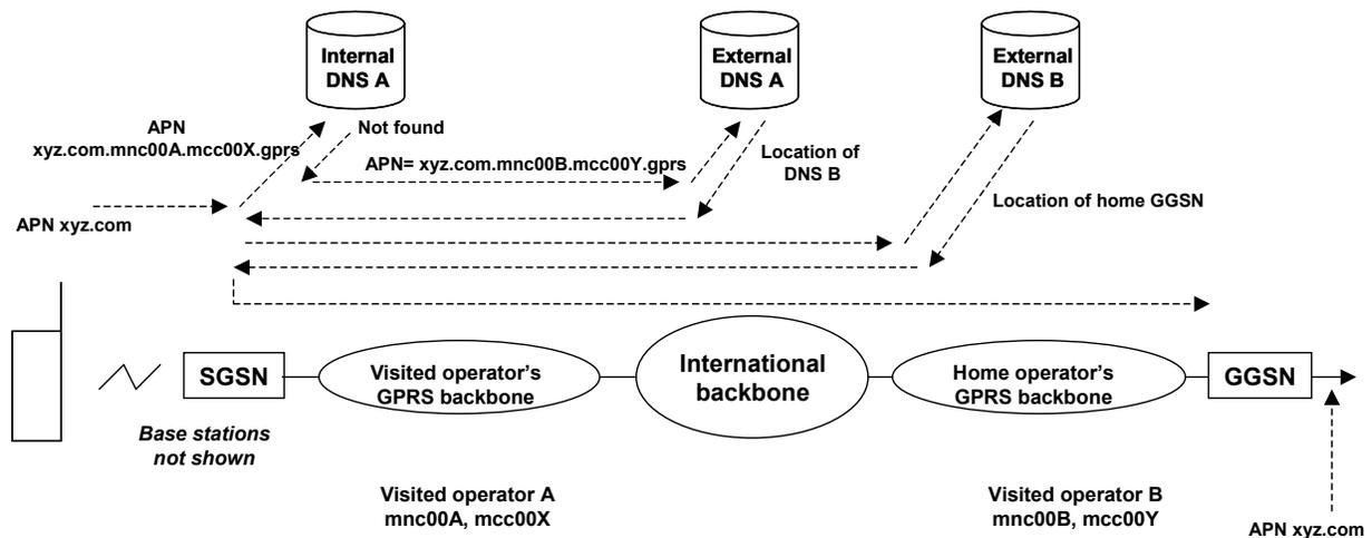
Figure 9: APN resolution and establishment of a GTP tunnel
