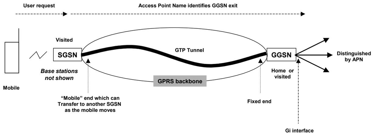
Figure 3: The GPRS access connection
