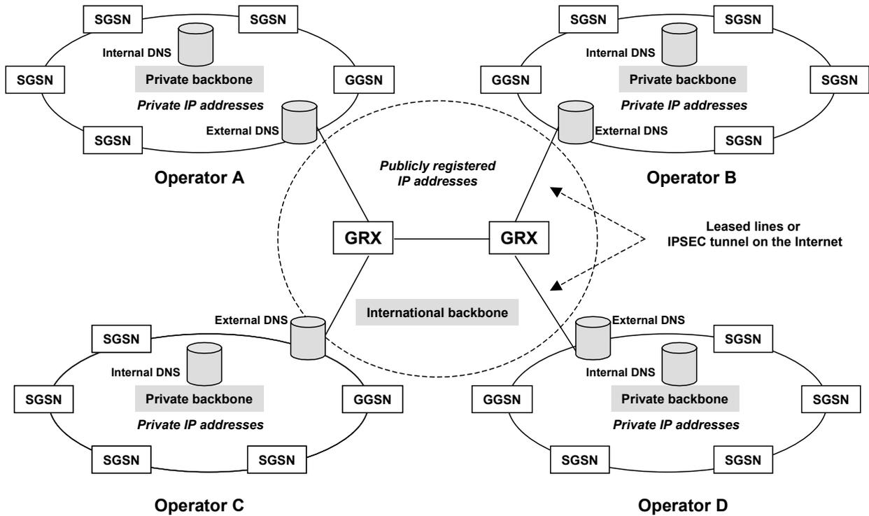
Figure 7: GPRS backbone arrangements
