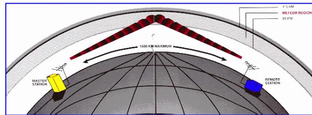
Data can consist of short messages such as sensor data readout, coded messages of up to several hundred characters, text messages of a few words or longer messages achieved by splicing together the transmission of successive bursts. In these applications, average throughput of up to several hundred words per minute are achieved with relatively simple equipment.
