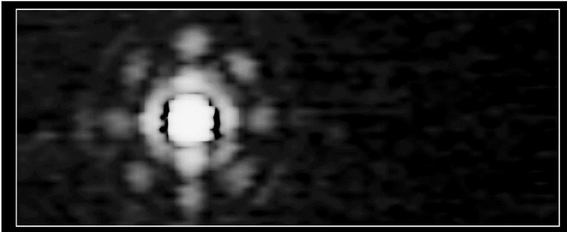
**Figure 1: Unpolluted measurement of the galactic object “3C84” in the 10.6-10.7 GHz band with the Effelsberg 100m radio telescope**
