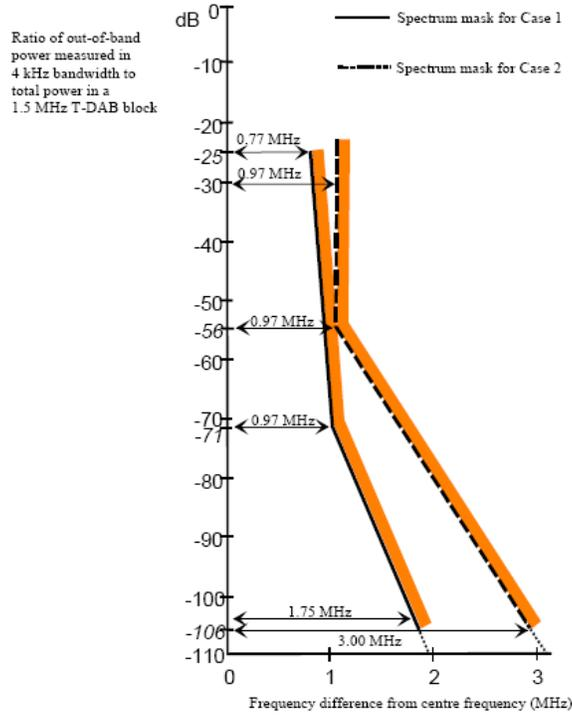
Figure 3.1: Spectrum masks for T-DAB out-of-band emissions
