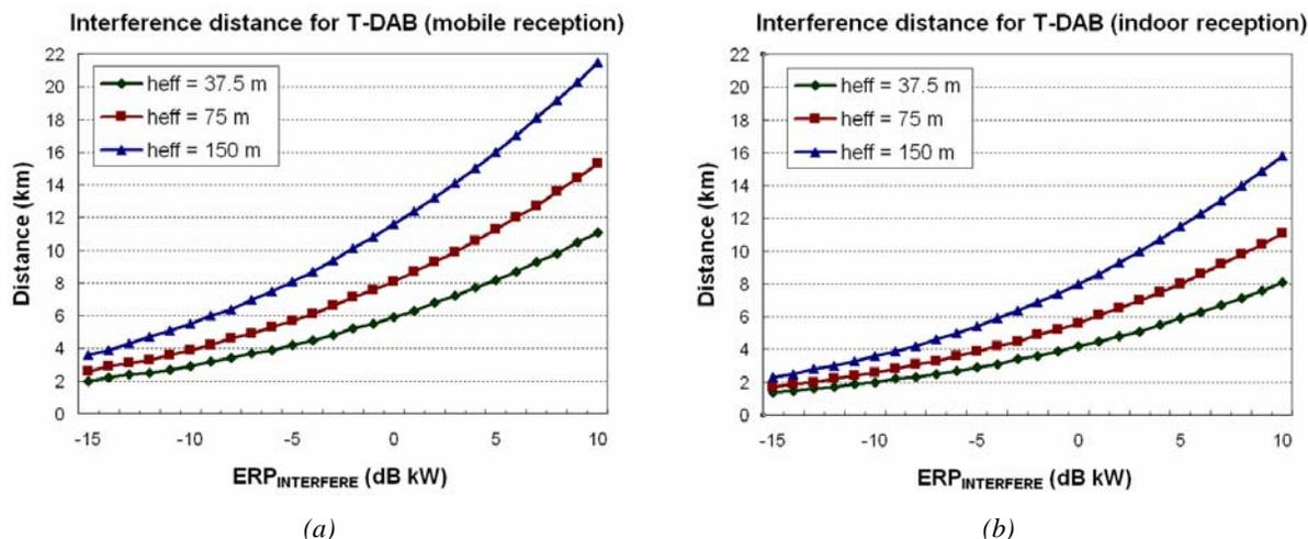
Figure 3.5: Minimum separation of a T-DAB interfering transmitter from the edge of a T-DAB transmitter coverage area for adjacent block interference: (a) mobile reception, (b) indoor reception
