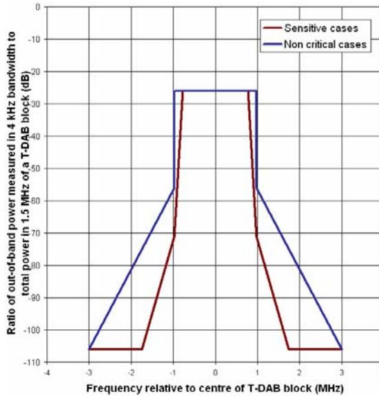
Figure 3.2: Spectrum mask for a single T-DAB frequency block
