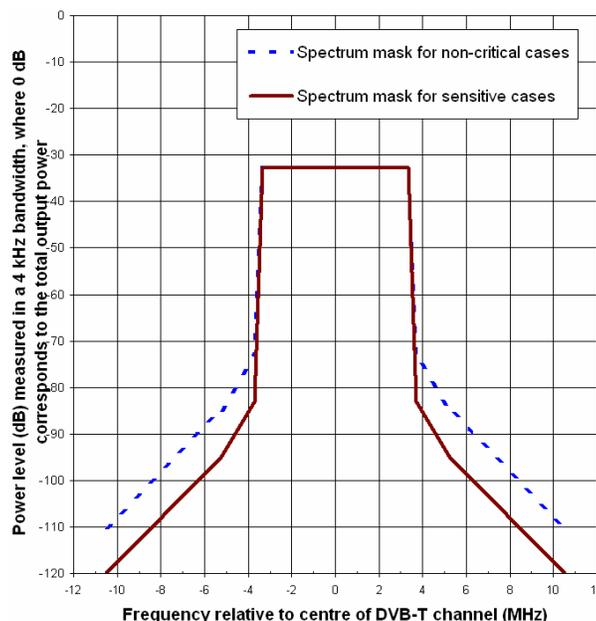
Figure 3.3: Spectrum mask for DVB-T in 7 MHz channel
