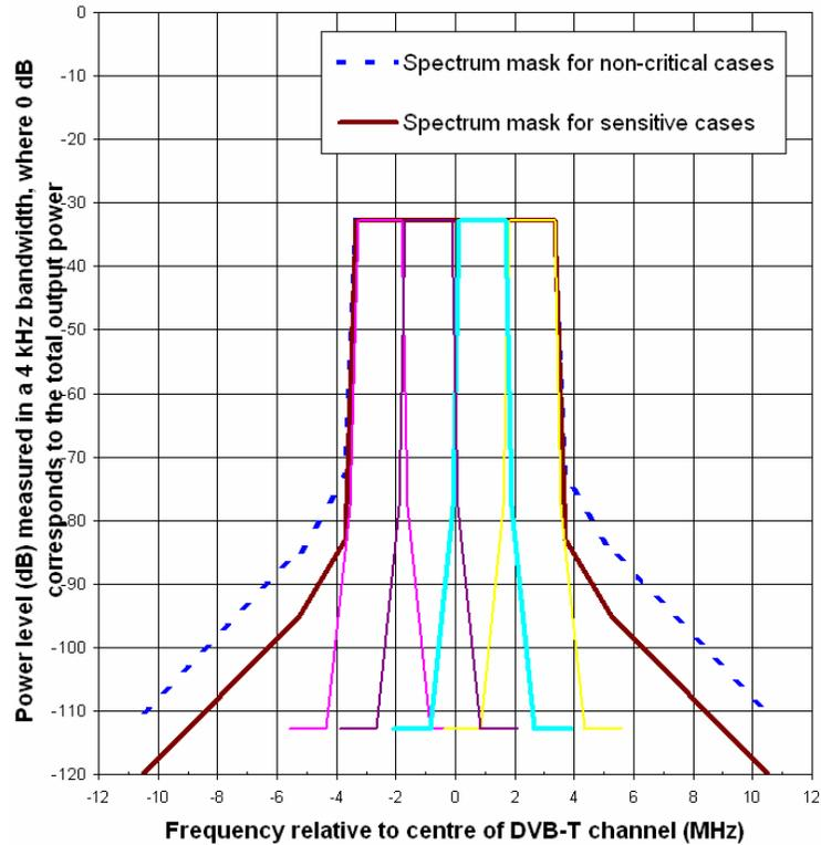
Figure 3.4: Spectrum mask for four aggregated T-DAB frequency blocks
